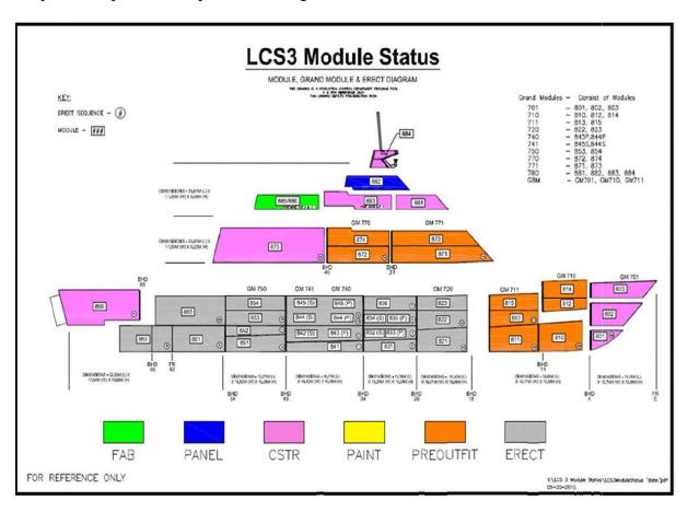
Def.'s Mot. Ex. H. The bow portion of the hull, comprised of Modules 801, 802, and 803, was still under construction. *Id.* Similarly, the transom, Module 866, to be secured to the stern
